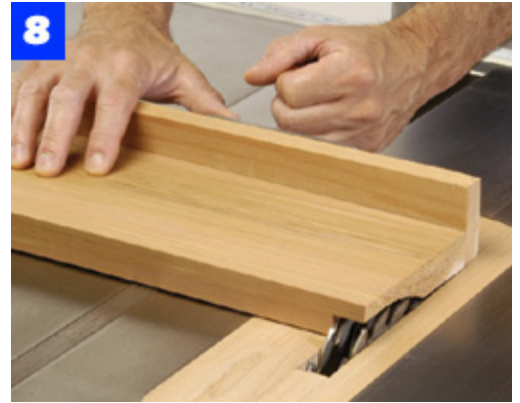
Use a dado blade to cut the chair rear-rail tenons. Note that these tenons are flush with the inner rail face.
