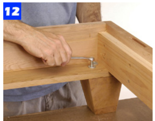
Fasten the feet by driving lag screws through the foot rails. Bore pilot holes to avoid splitting the feet.
