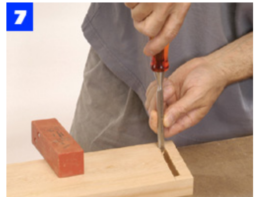
Use a sharp chisel to square the mortise ends. Since cedar is so soft, hand pressure is sufficient to cut the wood.
