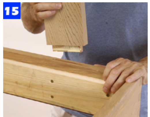
15 Spread glue in the side-rail mortises and on arm-post tenons. Join the parts and clamp to pull the joints tight.
