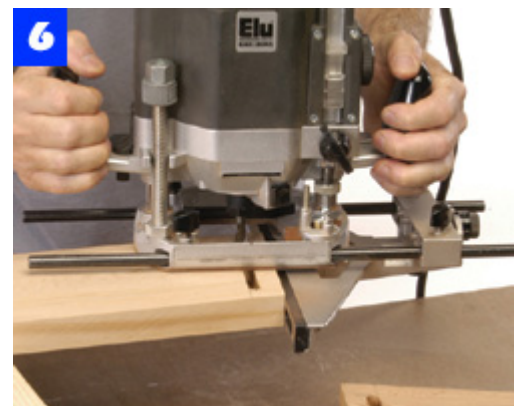
Rout the mortises in the chair side rails for the rear rail. Then, rout all mortises for the back assembly and arm posts.
