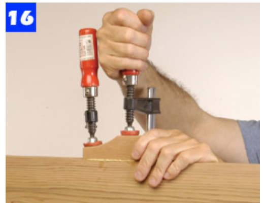
16 Cut the rear arm support blocks to shape, then glue them to the outside edges of the chair back.
