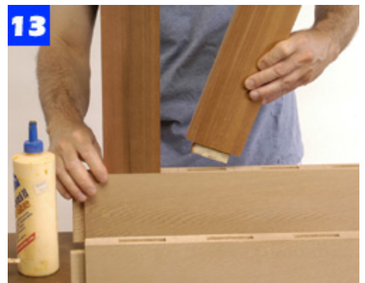
Glue the chair back slats to the back rails. When the glue is dry, apply glue and add the back stiles.
