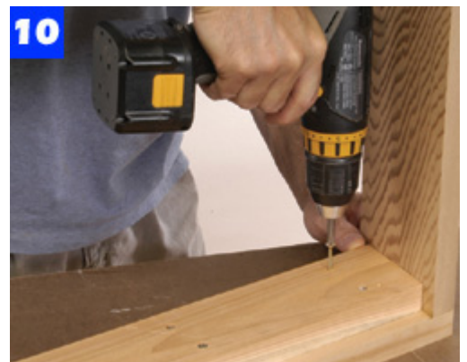
Cut the support cleats to size, and attach them to the sides of the chair and ottoman with galvanized deck screws.
