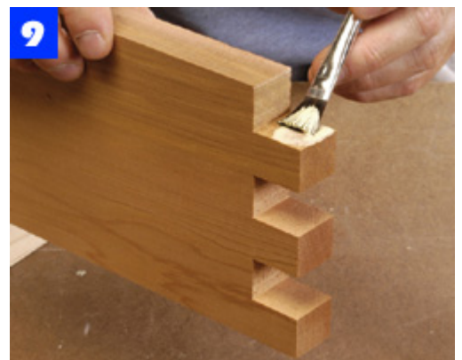
Apply glue and assemble the ottoman rails. For the chair, first assemble the rear/side joints, then add the front rail.
